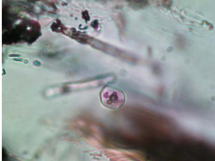
Fig.5. T=1150°C. View of melt inclusions in acid glass from plagioclase
